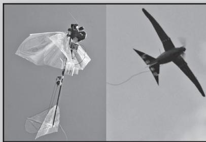
Fig. 2. Micro air vehicle "design" inspired by insect and bird flight. Left: DelFly. Right: RoboSwift.
