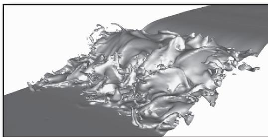
*Fig. 2. High fidelity simulation of a turbulent hydraulic jump with continuous breaking events. (Simulation by ME student, Milad Mortazavi)*
