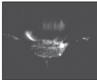
*Fig. 1. Microbubble cloud formed after a liquid-liquid impact event. The size of the impacting drop is about 5mm (Photo by ME students, Shahab Mirjalili and Lewis Marshall)*
