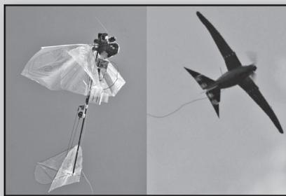
Fig. 2. Micro air vehicle "design" inspired by insect and bird flight. Left: DelFly. Right: RoboSwift.
